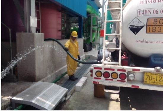
Picture1. tank field operator meet flexible host fall of the joint and sulfuric acid splash to driver and spilled to storm drainage and inform control room
